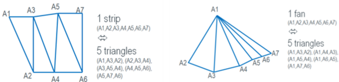
Figure 16: Examples of tessellated geometry for Number of Facets
