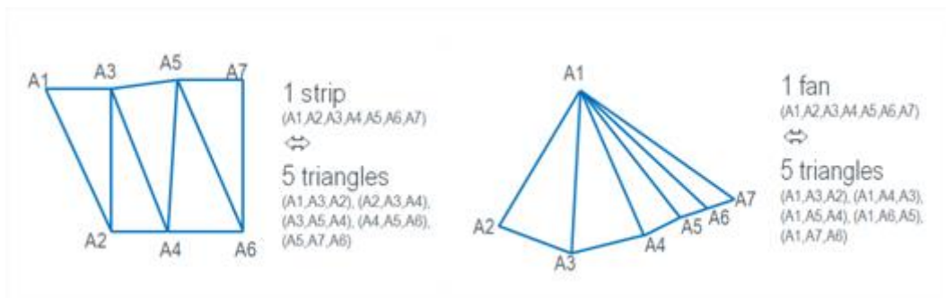
Figure 3: Triangle strips and triangle fans
