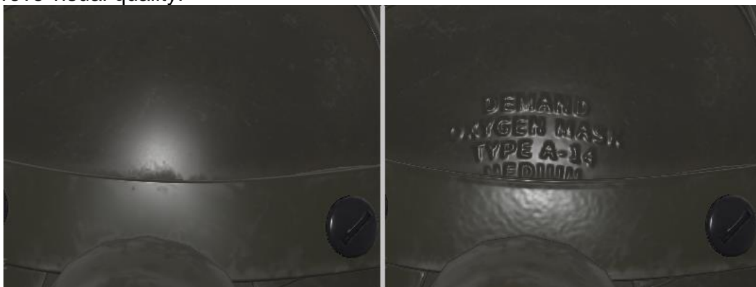
Normal texture may add extra details like scratches or imprints without altering geometry.
